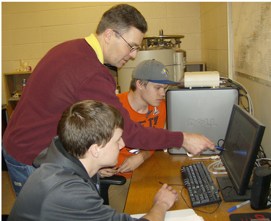
Kyle Schroeder (foreground) and Ryan Michel (background) are in the nuclear laboratory helping South Dakota State University Associate Professor Robert McTaggart calibrate the high-purity germanium detector for use in the gamma spectroscopy analysis of naturally occurring radioactivity in a soil sample. McTaggart started his second-straight NASA Summer Faculty Fellowship in May.
